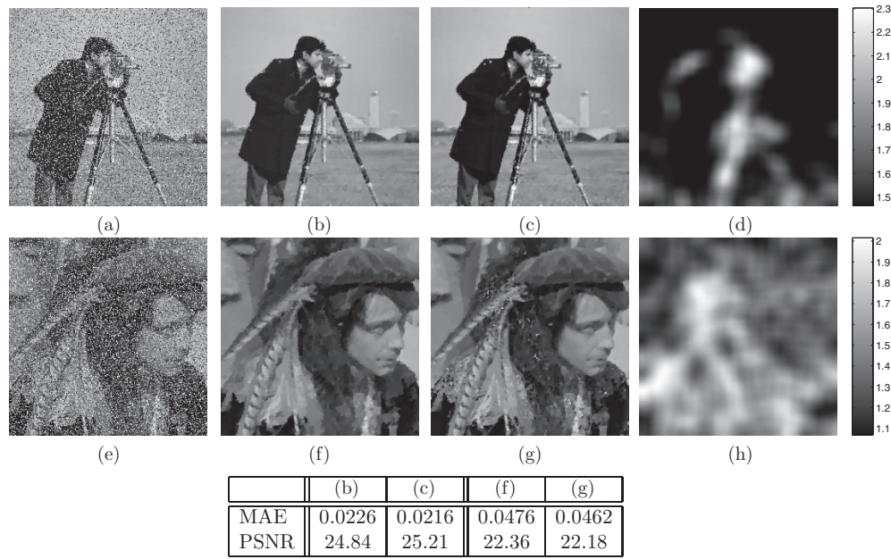
Figure 6. Cameraman : (a) image with random-valued impulse noise r = 0.4 , (b) denoising with the L^1 -TV model, \lambda = 1.3 , (c) denoising with the present method, (d) resulting \lambda . Man : (e) image with random-valued impulse noise r = 0.4 , (f) denoising with the L^1 -TV model, \lambda = 1.3 , (g) denoising with the present method and (h) resulting \lambda .
