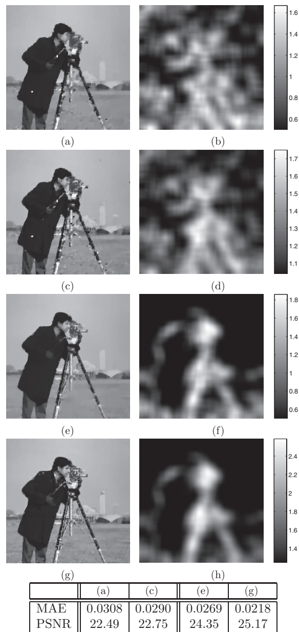
Figure 3. Salt-and-pepper noise: (a) restored image using algorithm (A), (b) resulting \lambda , (c) restored image using algorithm (B), (d) resulting \lambda . Random-valued impulse noise: (e) restored image using algorithm (A), (f) resulting \lambda , (g) restored image using algorithm (B), (h) resulting \lambda .
